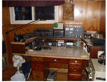
**EQUIP:** bottom left up and right: MFJ-4035 ps., Yaesu FT-2800 2m., Yaesu FT-847 6-2-hf xcvr., Yaesu-1000mp., Sp-6 spkr., Heath Ho-10 scope, Ameritron Al-80b, MFJ tuner, Rotor controls, Kenwood TS-820S.
