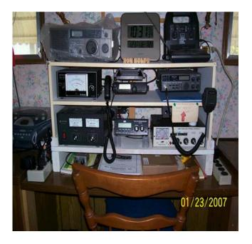
2 m Yeasu transceiver and a Radio Shack 10 m. transceiver. Below that is my power supply, an MFJ CW reader/keyer and a 10 m. antenna tuner. The small box with two knobs at the bottom left is a home-made 2 m. antenna tuner. If you enlarge this image you can plainly see the tuner (More about the tuner in a future article.)
